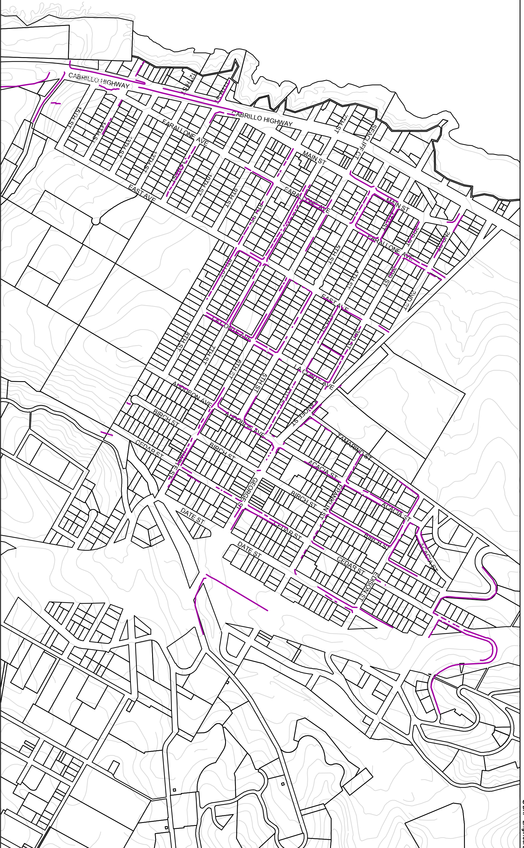
FIGURE 3A MIDCOAST STORM DRAIN INVENTORY AND ASSESSMENT EXISTING DITCHES WITH ADEQUATE CAPACITY (10-YEAR STORM EVENT) DRAINAGE REPORT
