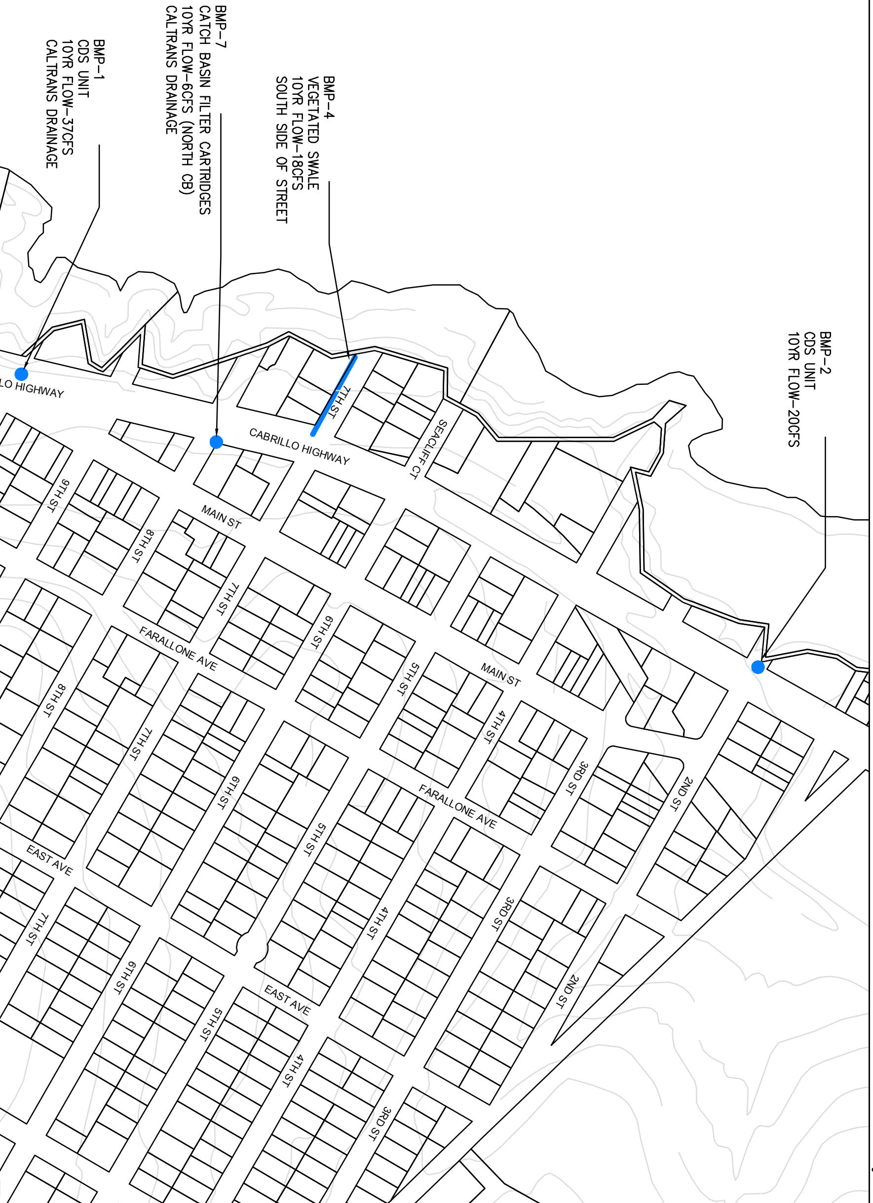
FIGURE 5A MIDCOAST STORM DRAIN INVENTORY AND ASSESSMENT PRIORITIZED OUTFALL BMP LOCATIONS DRAINAGE REPORT
